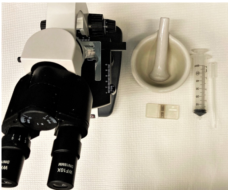
Figure 1. Nosema diagnosis equipment (mesh filter, water, and paper towel not shown)
